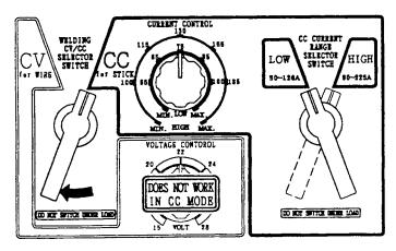
Figure 11. Welding Current Adjustment
